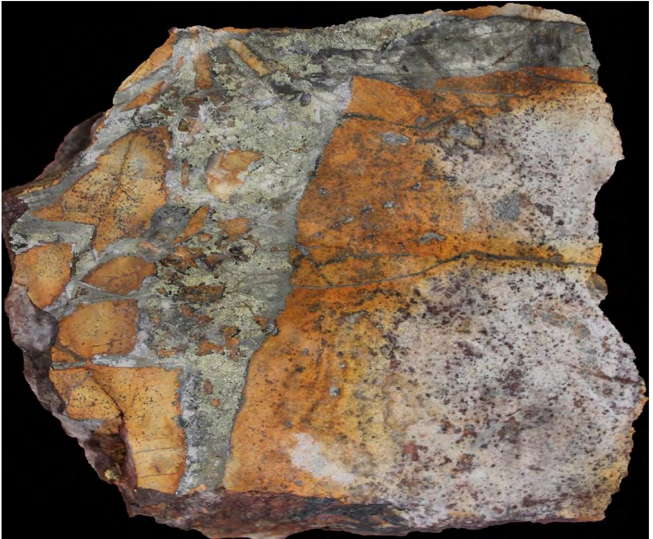
Photograph 4. Cut slab of breccia-veinlet stockwork in volcano-lithic sandstone from the southern part of the Dongil-Gunwi Mine. The sandstones contain abundant disseminated early stage ruby brown grains of sphalerite. The core of the breccia veins consist of pyrrhotite and chalcopyrite, with margin rims of the veins composed of galena and lesser black sphalerite (iron-rich species marmatite). Some of the chalcopyrite is being replaced by covellite-bornite. The orange coloration is an oxidation and feldspar alteration halo developed around the vein breccia composed of adularia. The observed mineralogy and alteration effects are consistent with reducing-oxidation interface conditions in a complex fluid mixing environment.
