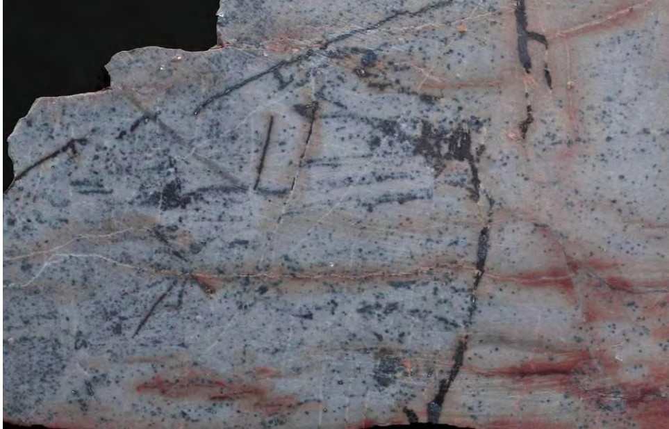
Photograph 2. Cut slab of hornfelsed siltstone with disseminated and very thin discontinuous fracture-filling base metal sulphide veinlets, collected from the northern part of the Dongil-Gunwi Mine. Sample No 242716; 27g/t Ag, 905ppm Cu, 1.59% Pb, 1.13% Zn, 0.45% As, 13 ppm Bi, 44ppm Sb and 6.08% Fe as pyrrhotite.
