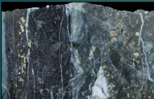
Chalcedony-actinolite-magnetite vein, breccia comb quartz, carbonate & sulphides, Haman. # 243319: 1.99g/t Au, 9g/t Ag, 1.10% Cu, 186ppm Bi.
