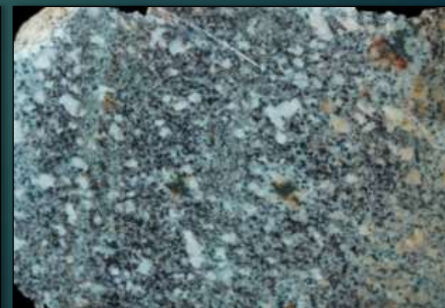
Secondary biotite altered Monzonite porphyry, Okbang. # 243306: 0.34g/t Au, 0.22% As, 109ppm Co.
