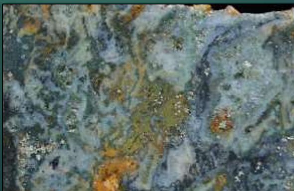
Breccia with quartz, magnetite, sulphide bands and hypogene jarosite, Haman. # 243323. 0.47g/t Au, 26g/t Ag, 1.25% Cu, 0.16% As, 109ppm Bi, 9.08% Fe.
