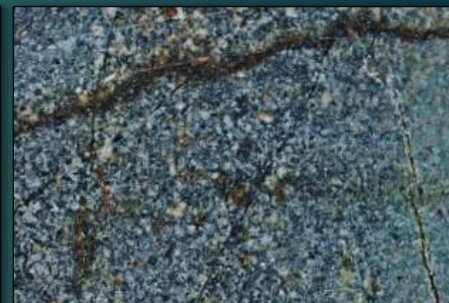
Monzonite with secondary biotite-magnetite alteration and sulphide-magnetite veinlets, Gilgok. # 243331: 0.20g/t Au, 830ppm Cu, 5.40% Fe.
