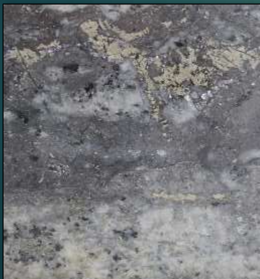
Silica-sulphide breccia, Goroseoksan. Sample 155507: 2.93g/t Au, 159g/t Ag, 9.32% Cu, 1.43% Pb, 3.06% Zn, 0.22% Sb.
