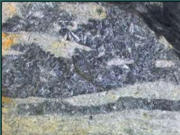
Radiating prismatic crystals of tremolite/scapolite? in volcaniclastic, Okbang. # 243310; 710ppm Ba.
