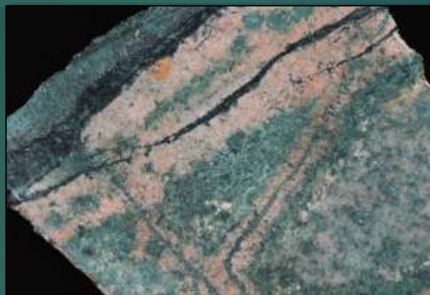
Tourmaline-magnetite veinlets with K-feldspar rim and chlorite altered Monzonite, Haman. # 243318: 519ppm Cu, 13ppm Mo, 7.56% Fe.
