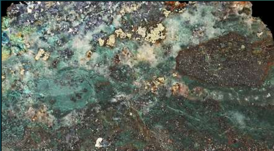
Comb quartz vein stockwork, Ogsan. # 155579: 0.11g/t Au, 140g/t Ag, 0.90% Cu, 2.31% Pb, 2.82% Zn, 0.15% Mo, 388ppm Bi, 215ppm W.
