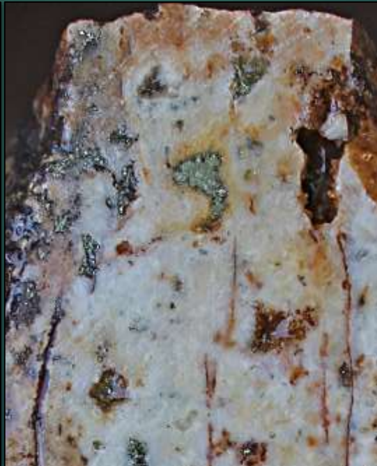
Quartz vein, Gunbuk Main Vein; # 243402: 6.05g/t Au, 28g/t Ag, 1.14% Cu, 0.32% As, 554ppm Bi, 8.31% Fe
