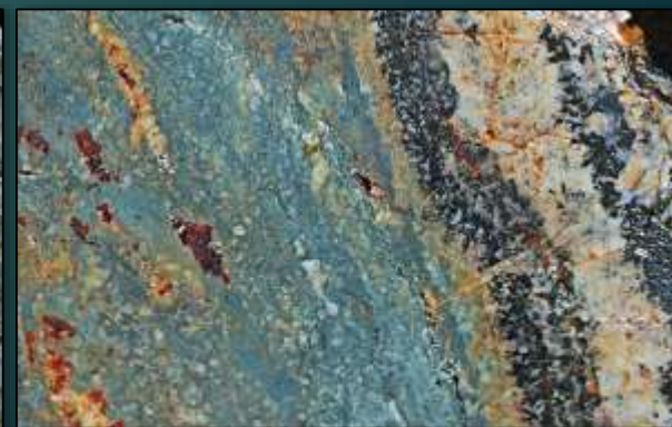
Quartz-magnetite-actinolite vein in chlorite-epidote-quartz altered monzonite, Oguk. # 243373: 1.47g/t Au, 15g/t Ag, 0.38% Cu, 0.11% As, 60ppm Bi, 11.05% Fe.
