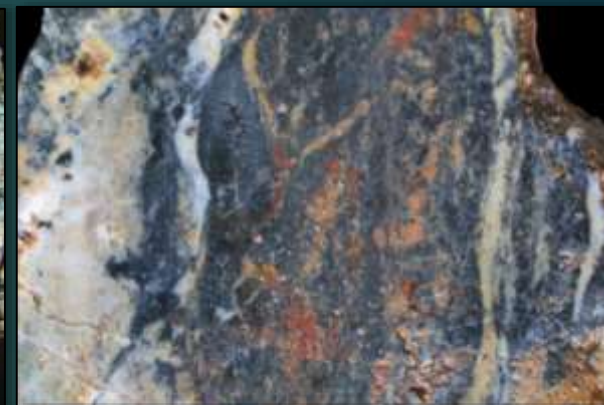
Quartz-magnetite-specularite-carbonate vein, Namgok. # 243343: 0.86g/t Au, 5g/t Ag, 924ppm Cu, 10ppm Mo, 9.07% Fe.
