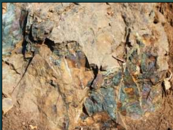
Silica-pyrite hornfelsed siltstones with quartz veinlet stockworks, Bukgok. # 243360; 0.27g/t Au, 7g/t Ag, 0.38% Cu, 74ppm Mo.
