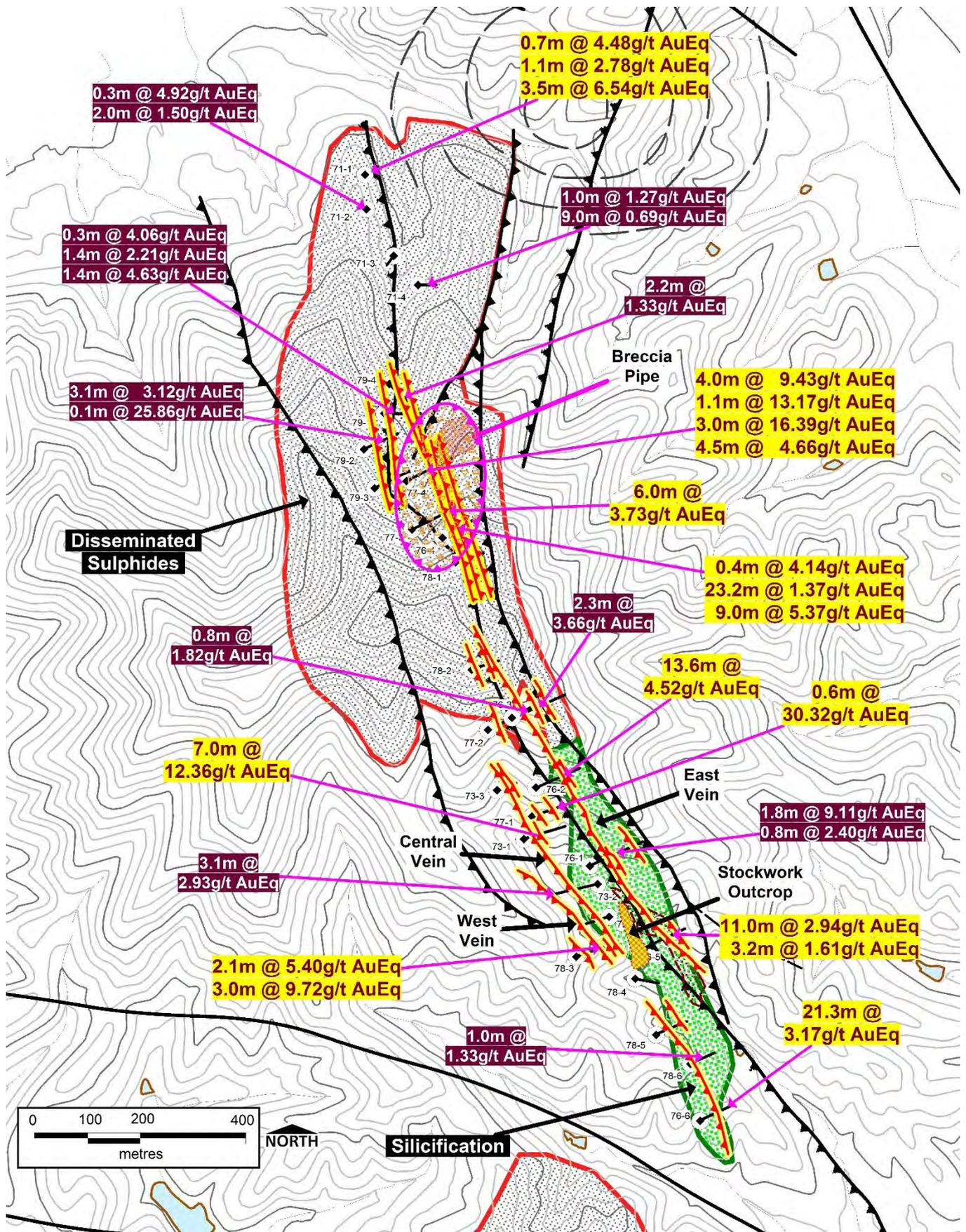
Digital Topographic Map of Dongil Prospect, showing historical drillholes and Mineralized Intersections (AuEq). Sub-surface alteration is also shown, including disseminated sulphides in the rhyodacite and sandstone, as well as fault-vein-related, typically high-temperature skarn/hornfels/silicification in the southern part of the fault system. Mineralization has not been closed off and remains open in all directions.
