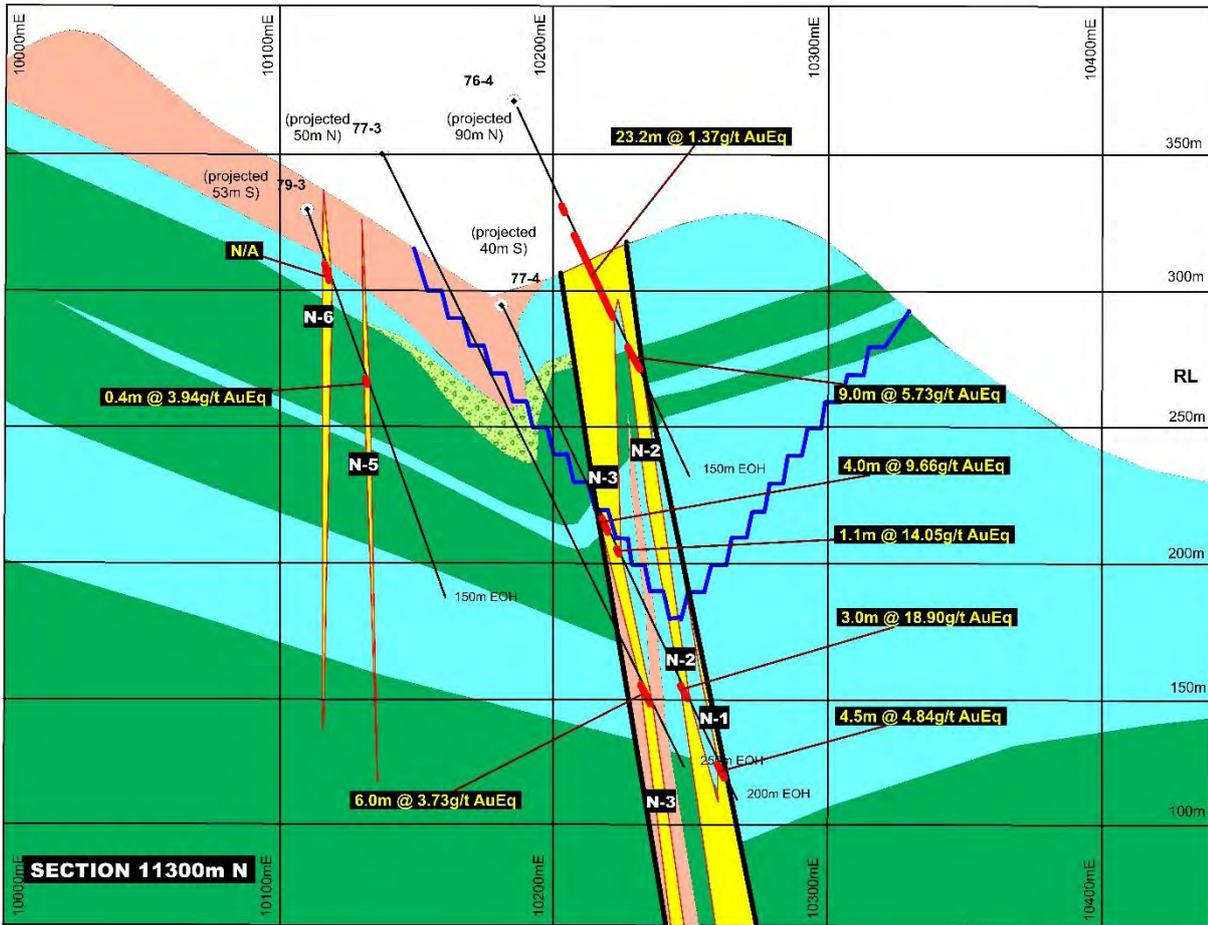
Dongil North, Drill Section 11200mN. Note numerous quartz-sulphide veins recorded but not assayed (N/A). A conceptual open pit outline is shown using 10m bench heights at 60°.
