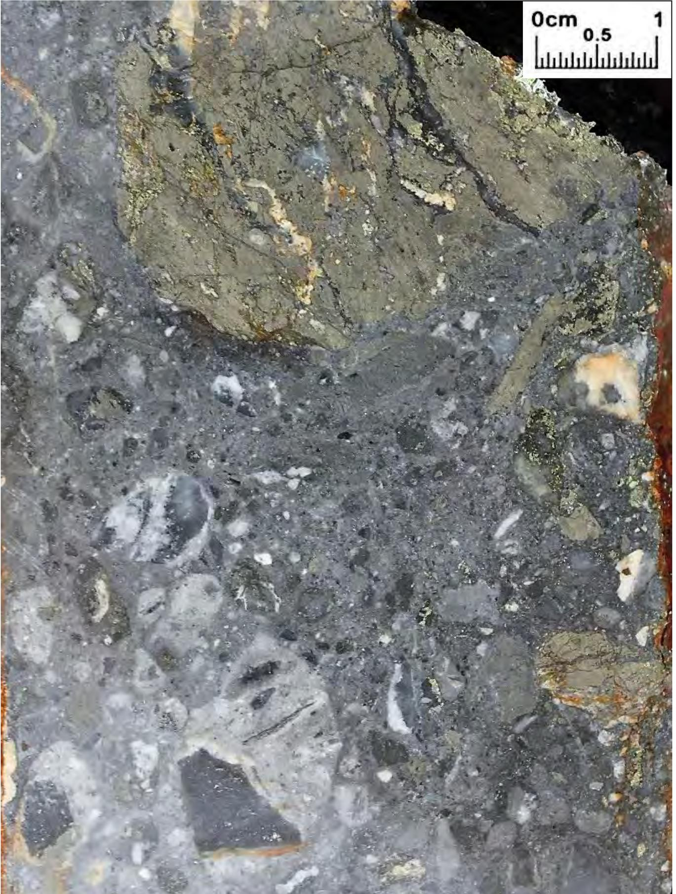
**Mineralized hydrothermal breccia, West Vein at Dongil South.** The entrained clasts of bedded massive sulphide (pyrrhotite-pyrite-chalcoprite), sediments and quartz-carbonate veins are cemented in a finer matrix of rock flour, sulphides (pyrite, chalcopyrite) and comb quartz, clearly indicating multiple episodic phases of mineralization. Sample 155502: 0.28g/t Au, 86g/t Ag, 0.94% Cu, 0.83% Zn, 0.35% Pb, 0.23% Sb, >500ppm Sn, 195ppm Co, 0.64% As.
