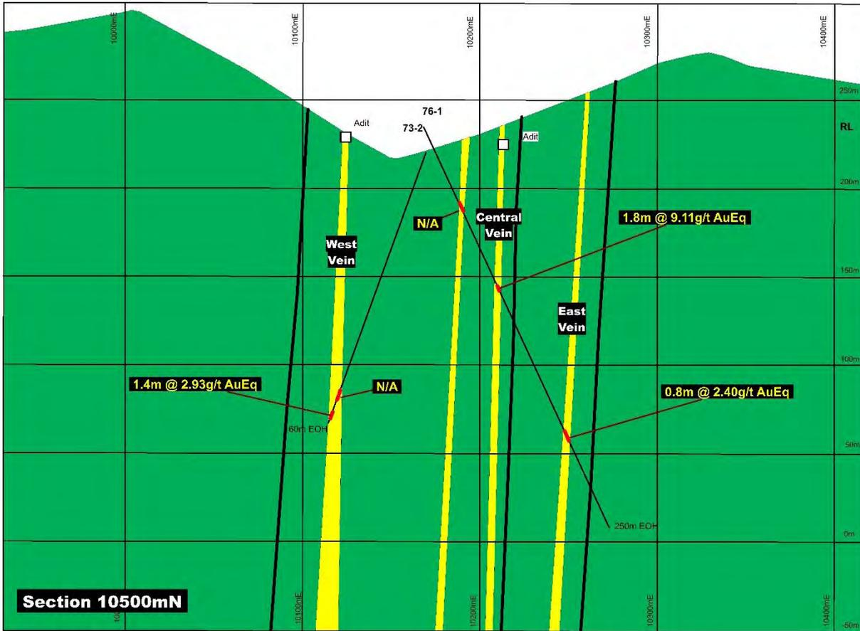
Dongil South, Drill Section 10500mN. Note numerous quartz-sulphide veins recorded but not assayed (N/A).
