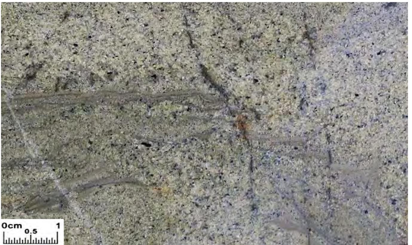
**Tuffaceous volcanoclastic sandstone of the Sagok Formation, Dongil North adit.** Soft sediment compaction features, micro-faulting displacement of thin silty beds, along with disseminated and diffuse sulphide-lined fractures provide some evidence of syn depositional mineralization. Sample No 242718; 0.17% Zn, 0.19% As, 30ppm Sb.
