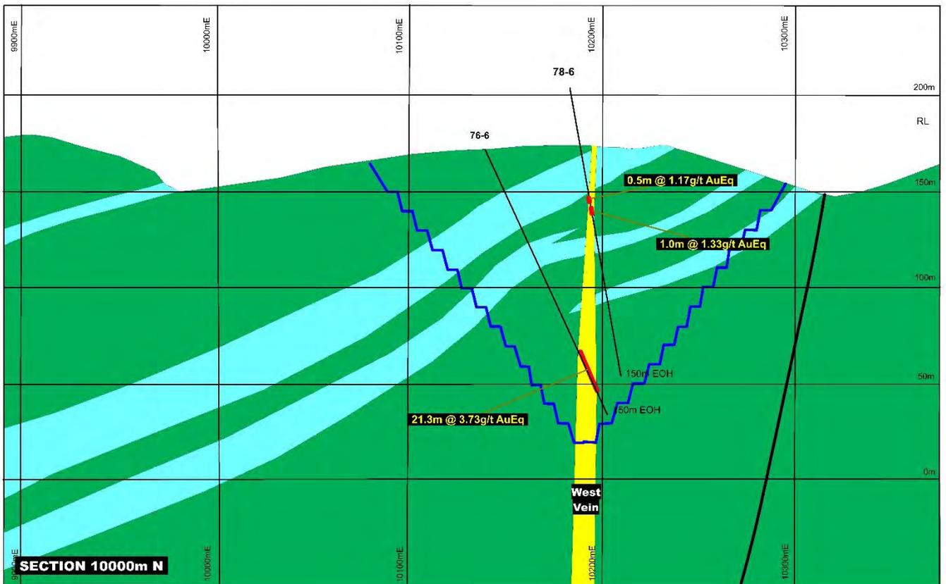
Dongil South, Drill Section 10000mN. Lack of drilling is evident and required to the east. There is an unexpected very wide vein at the southern end of Dongil which needs follow up drill testing. A conceptual open pit outline is shown using 10m bench heights at 60°.
