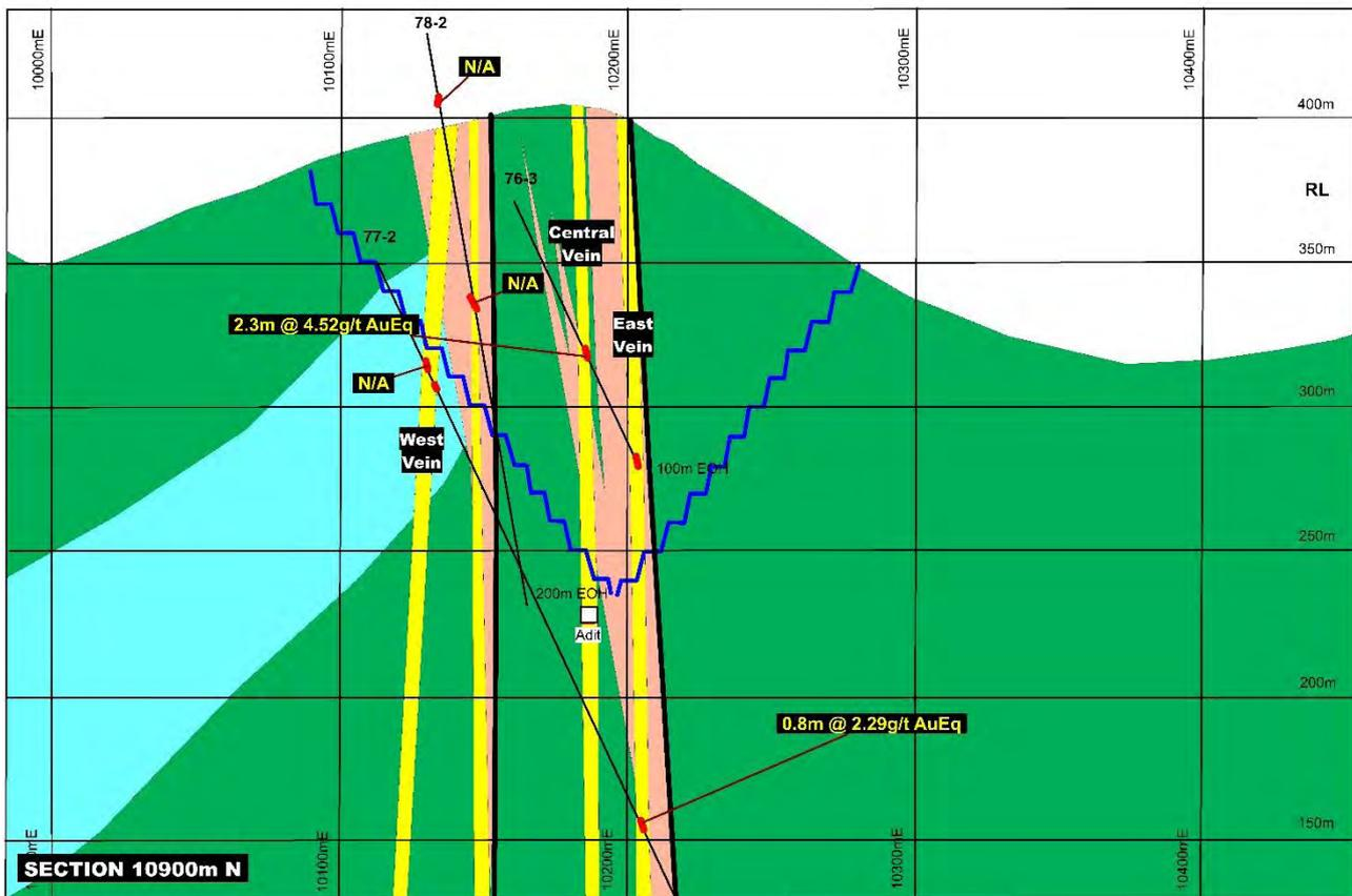
Dongil North, Drill Section 10900mN. Note numerous quartz-sulphide veins recorded but not assayed (N/A). A conceptual open pit outline is shown using 10m bench heights at 60°.
