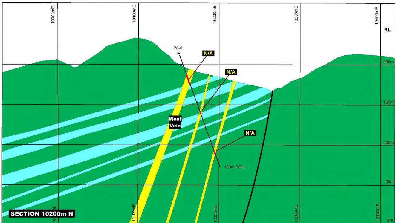
Dongil South, Drill Section 10200mN. Note numerous quartz-sulphide veins recorded but not assayed (N/A). A lack of drilling is evident on this section and further drilling is required to the east.
