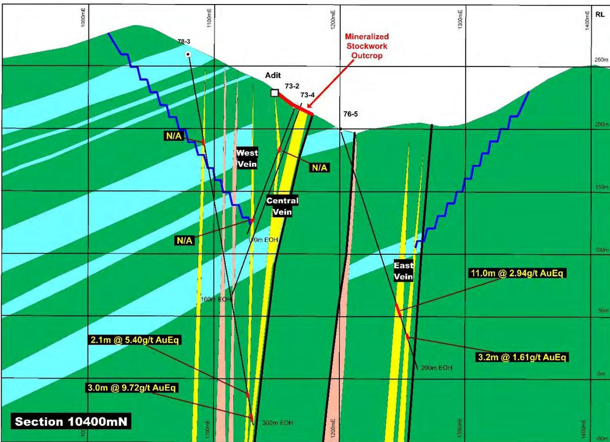
Dongil South, Drill Section 10400mN. Note numerous quartz-sulphide veins recorded but not assayed (N/A). A conceptual open pit outline is shown using 10m bench heights at 60°.
