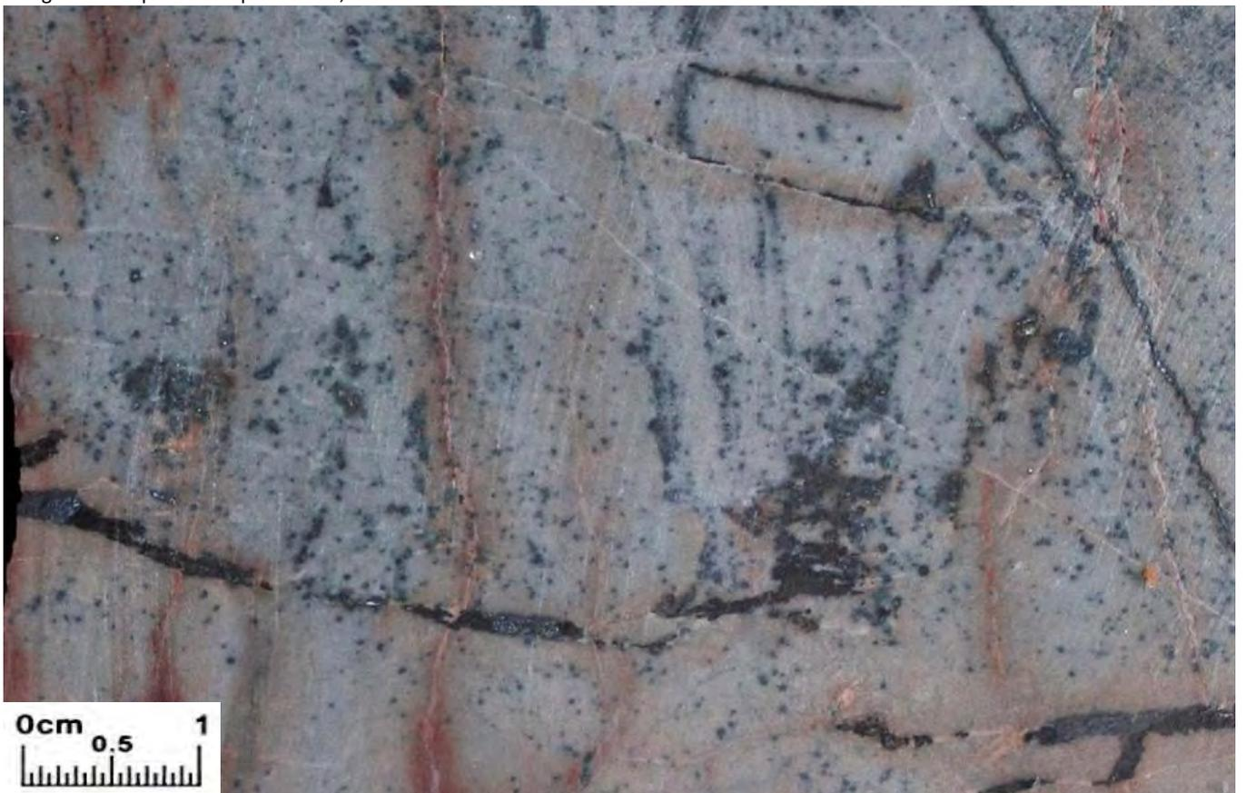
**Rhyodacite with disseminated and thin discontinuous fracture-filling base metal sulphide veinlets, Dongil North adit.** Sample 242716; 27g/t Ag, 905ppm Cu, 1.59% Pb, 1.13% Zn, 0.45% As, 13 ppm Bi, 44ppm Sb & 6.08% Fe as pyrrhotite. This sample clearly illustrates the potential of the rhyodacite dome intrusion to host bulk tonnage disseminated mineralization.
