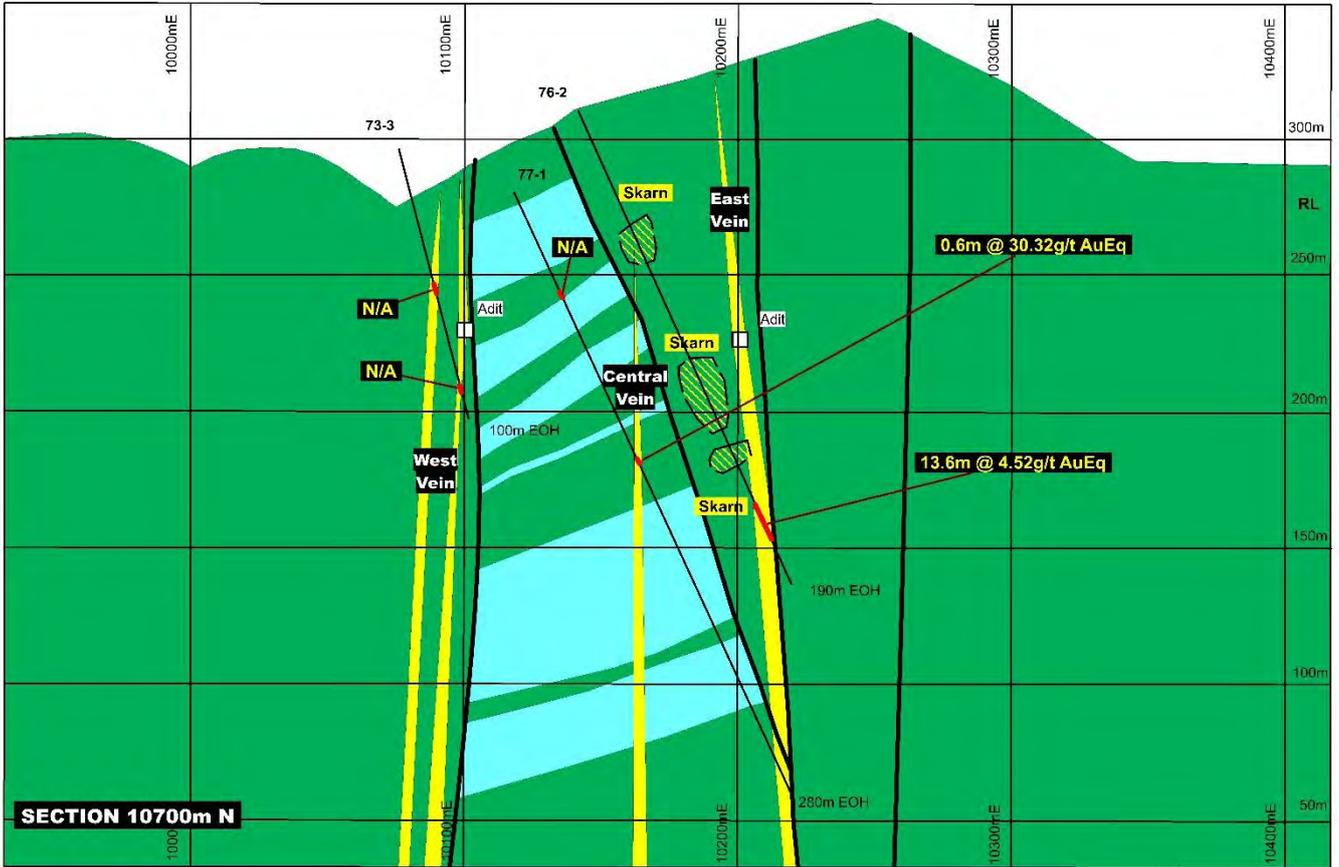
Dongil South, Drill Section 10700mN. Note numerous quartz-sulphide veins recorded but not assayed (N/A).
