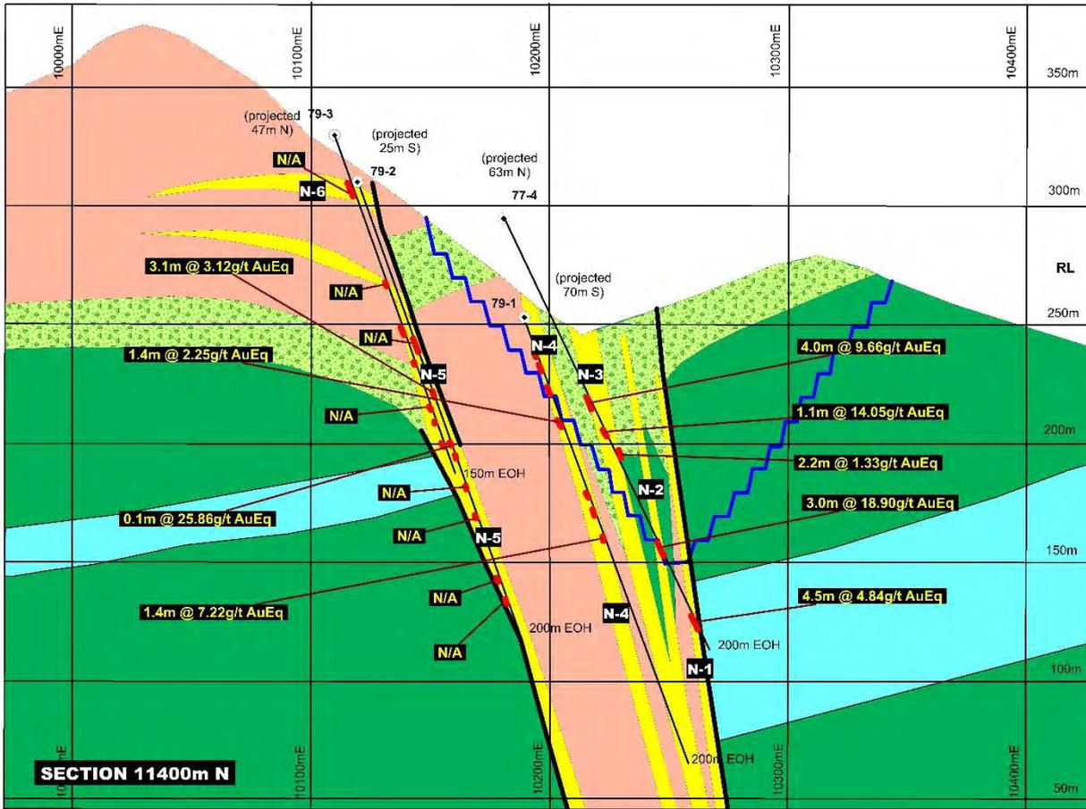
Dongil North, Drill Section 11400mN. Note numerous quartz-sulphide veins recorded but not assayed (N/A). A conceptual open pit outline is shown using 10m bench heights at 60°.
