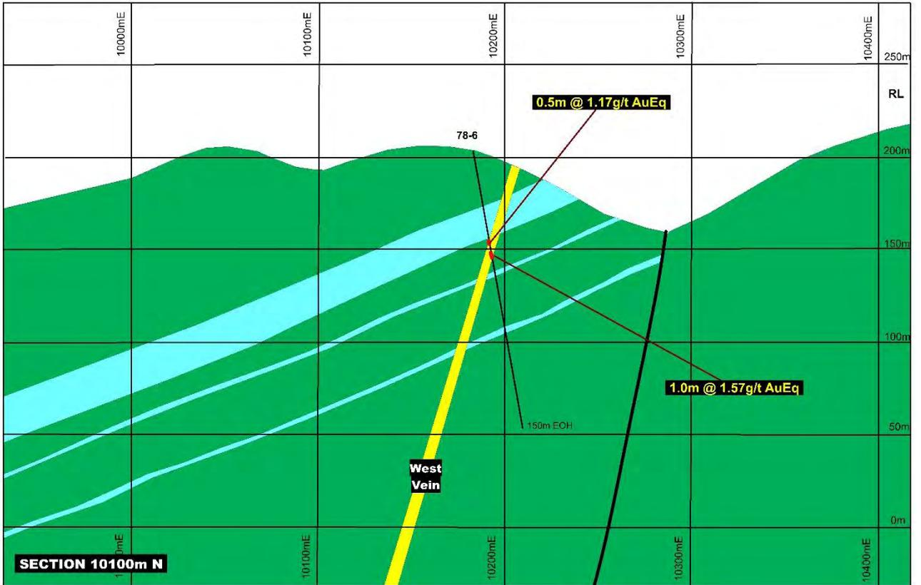
Dongil South, Drill Section 10100mN. Lack of drilling is evident on this section and further drilling is required to the east.
