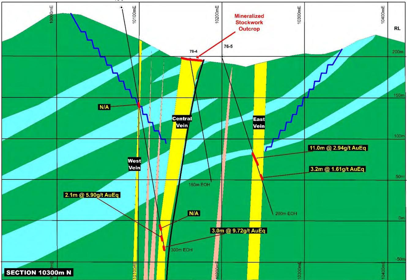
Dongil South, Drill Section 10300mN. Note numerous quartz-sulphide veins recorded but not assayed (N/A). A conceptual open pit outline is shown using 10m bench heights at 60°.
