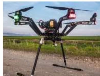
Flying at low altitude (30m) with the bird on a 10m tow line, at a minimum speed of 10m/s to minimize drag, a c-drone UAV can cover ground 6-10 times faster than a walking operator, in all types of terrain, be flown at night, in poor visibility conditions, and over dangerous topography.
