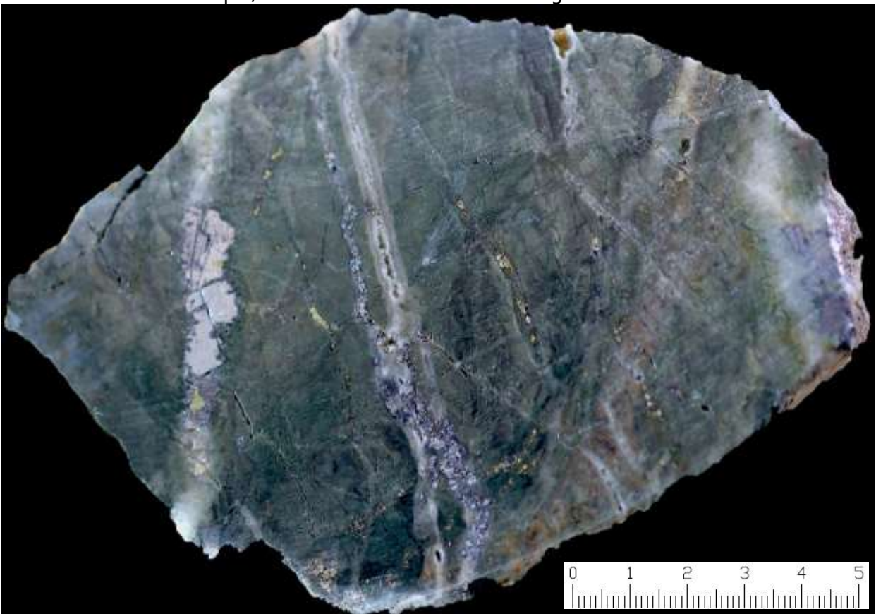
Sample 00009, Buk Adit. Sheeted stockwork quartz-sulphide veinlets hosted in silicified/hornfelsed siltstone (mapped by KMPC as "chert"). Visible galena, sphalerite and chalcopyrite. Assays pending.
