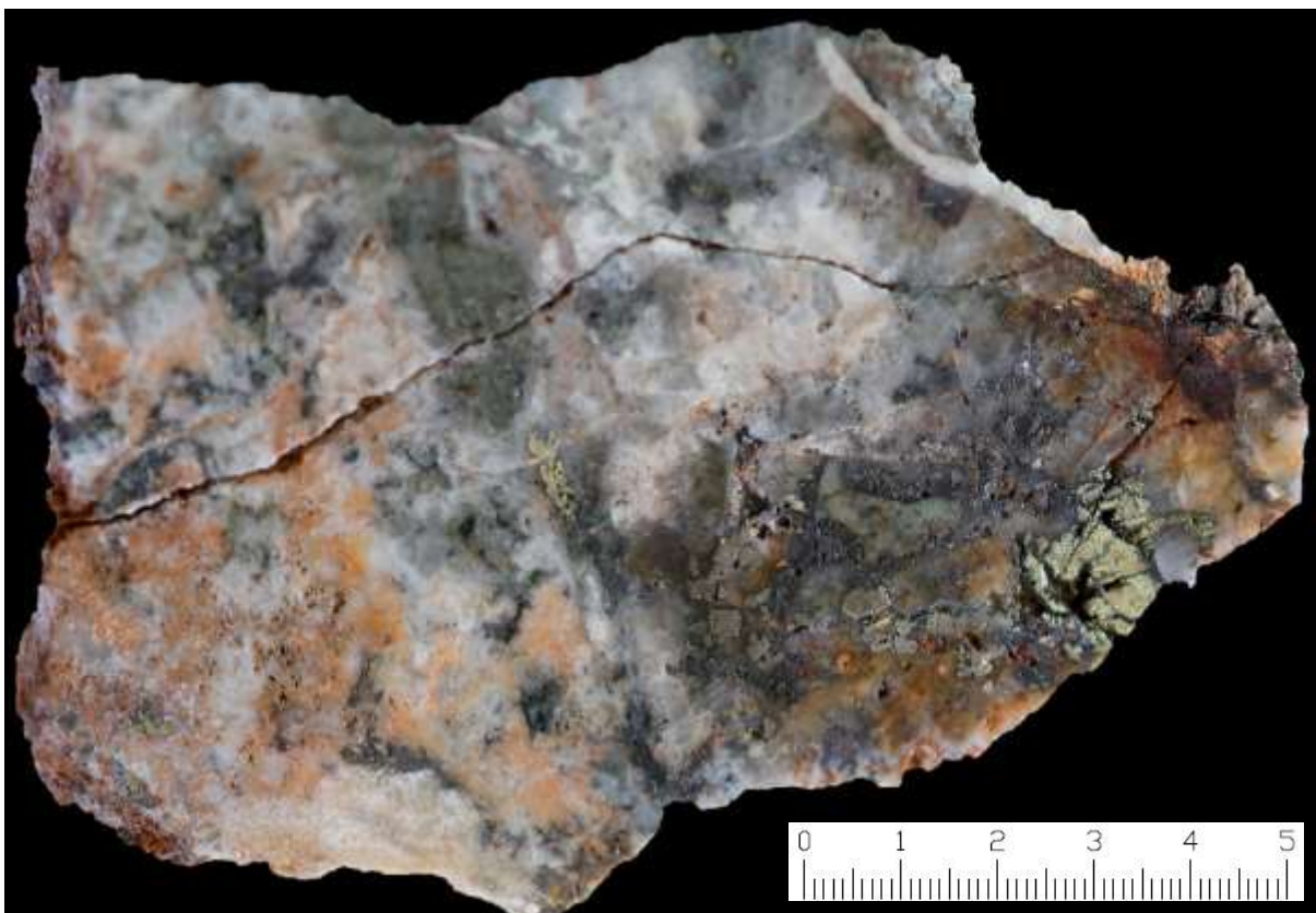
Uiseong Project - Kyungwha Mine. Sample 00006. Epithermal vein textures in quartz-adularia vein. Adularia is an indication that “boiling” has occurred and is a positive sign for elevated gold grades. Visible chalcopyrite, galena and sphalerite. Assays pending.
