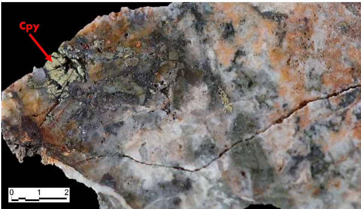
Photograph 18. Epithermal vein breccia, with "jigsaw" quartz (cloudy white), chalcedony (light grey), adularia (pink) and sulphides (dark grey), Jukdong adit (chalcopyrite grain shown in red). Sample No 00006: 0.25g/t Au, 345g/t Ag, 1.11% Cu, 1.47% Pb, 0.16% Bi & 73ppm Sb.
