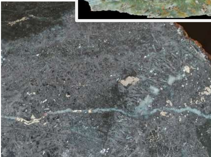
Photograph 12 (left). Magnetite-hematite skarn (note blades of specular hematite) with crosscutting quartz-chalcopyrite veinlet, Dundok Adit. Sample 242733: 0.12% Cu, 118ppm Mo, 2.52ppm Ge, 870ppm W.
