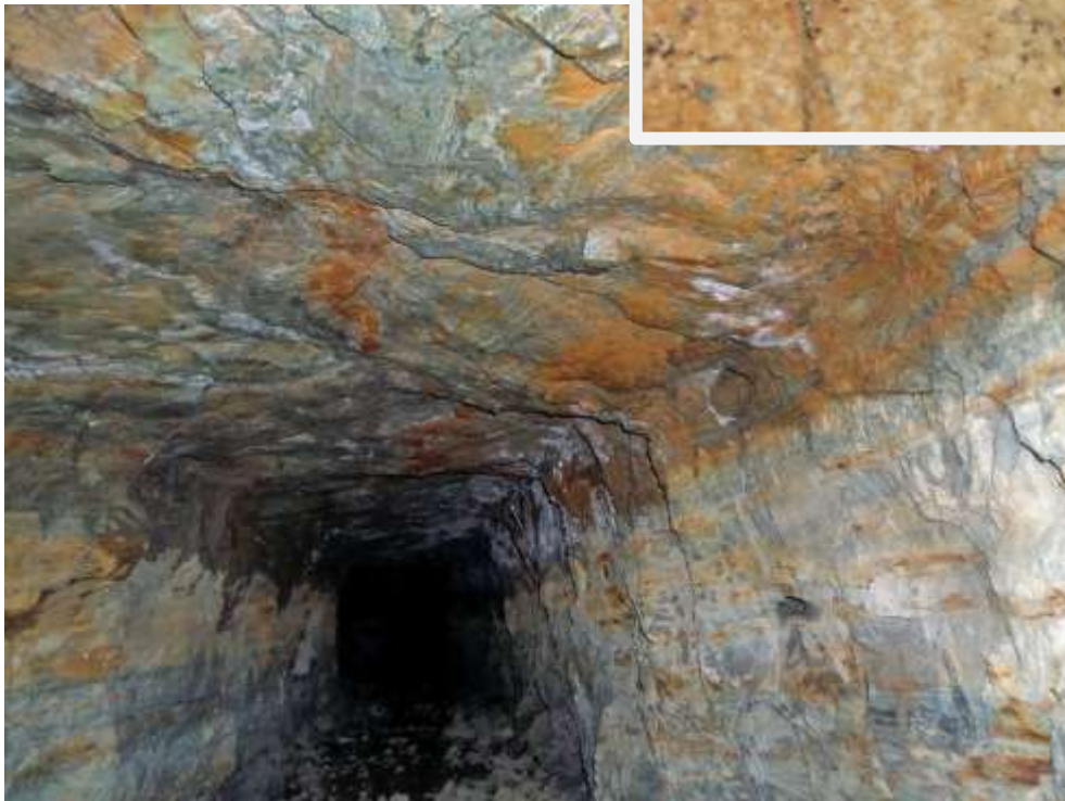
Photograph 6 (above). View inside the Ilkwang Adit. Mineralised carbonatite dyke and vein breccia exposed in the roof (see inset) and bands of disseminated, replacement style mineralisation in the surrounding flat-lying wall rock sediments indicate both high-grade and bulk tonnage potential.
