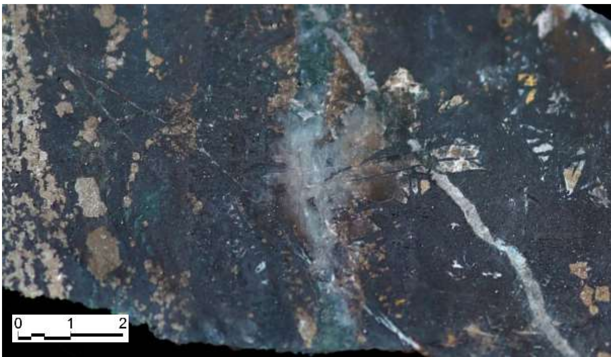
Photograph 3. Close up of fluidised, banded pyrite-magnetite-chlorite-quartz carbonatite breccia from the Main Adit, Sample 00002: 0.58g/t Au, 206ppm Co, 0.13% Cu, 274ppm Mo, 1.82ppm Ge, 121ppm W.
