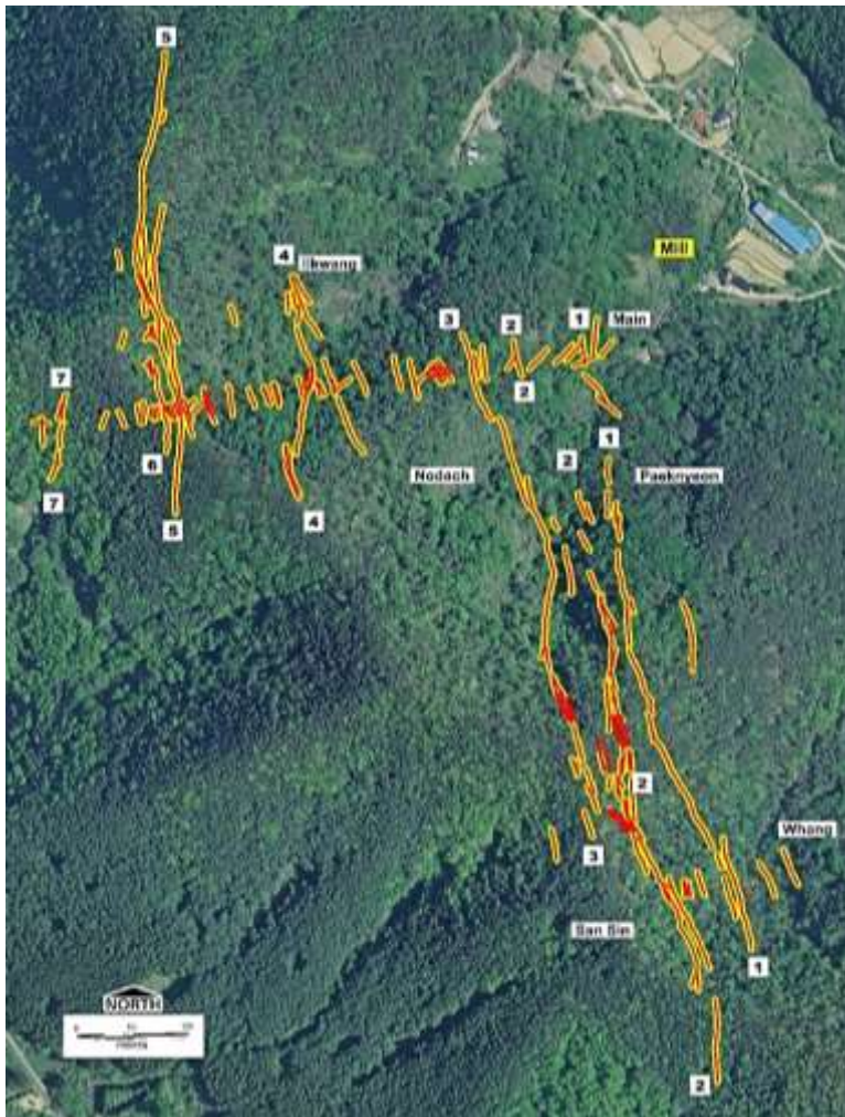
Figure 1. Aerial View of Jaeilgunbuk with vein system superimposed, adit portals and the old mill shown.
