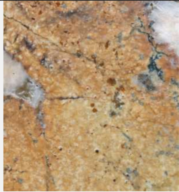
Photograph 5 (below). Close up of mineralised carbonatite dyke, Ilkwang Adit, Sample 155890: 0.34g/t Au, 0.55% As, 2.44% Mn, 103ppm Bi, 111ppm Co, 497ppm Cu.
