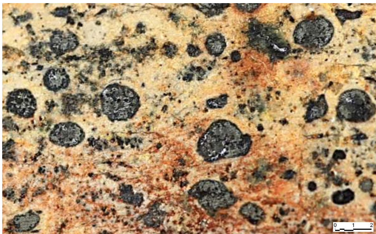
Photograph 1. Sulphide spherulites (1-3mm diameter) entrained in the rhyodacite dyke associated with the Dongil West mineralised structure. The ovoid-shaped sulphide spherulites (“raisin toast” texture) are rarely observed and strongly indicate a magmatic sulphide source-origin. This implies the dyke could be connected to an underlying larger mineralised intrusion at depth. Sample 00020: 32g/t Ag, 837ppm Cu, 1.67% Pb & 0.99% Zn.
