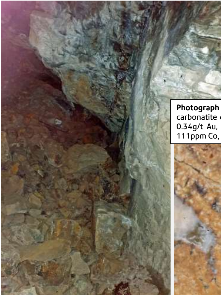
Photograph 4 (left). View looking north inside the Nodach No 1 Adit along the strike of the mineralised breccia, with entrained carbonatite dropped to floor (probably by airleg hand-drill and blast). An ultramafic (serpentinite) dyke is exposed in the footwall at right. The ultramafic dyke is likely related to the layered gabbro intrusion.
