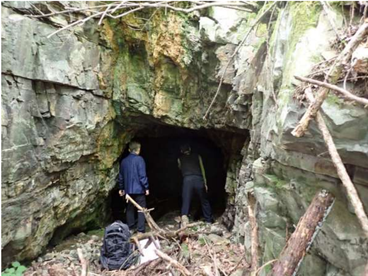
Photograph 17. The unrecorded adit located east of Jukdong North, shown by a local resident (right) to the Registered Geologist (left). A 2-metre wide, subvertical, sulphide-quartz-clay vein breccia structure is evident in the adit roof. The surrounding wall rocks are composed of argillic clay altered, gently-dipping purple-green siltstones and mudstones of the Sagok Formation.
