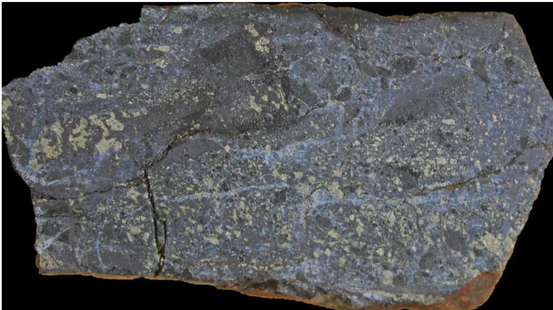
Haman Project - Dundok Adit dump. Sample 242734-1: 0.19g/t Au, 7g/t Ag, 250ppm As, 409ppm Co, 0.37% Cu, 14ppm Ga, 0.44ppm Ge, 63ppm Mo, 32.90% Fe. Very dense, heavy magnetite-specular hematite skarn with disseminated very fine sulphide matrix breccia. Enhancement of the image shows wispy, ghost-like blue-grey quartz/silica matrix indicating the early breccia is overprinted by a fluidizing colloidal quartz stage. Entrained breccia clasts-fragments are evident, along with chalcopyrite, pyrrhotite, pyrite and arsenopyrite grains.
