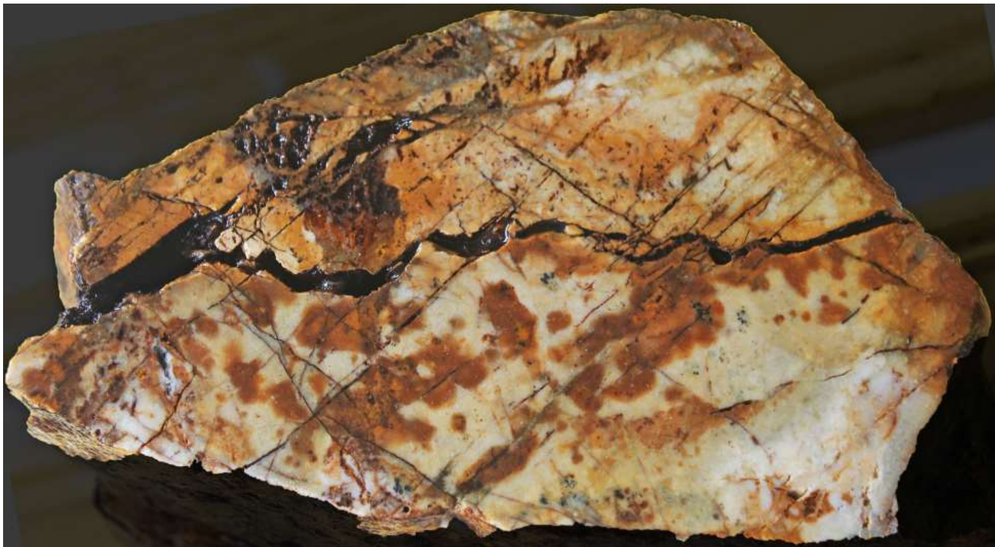
Haman Project - Okbang Adit dump. Sample 242736: 0.05g/t Au, 0.30% As, 110ppm Cu, 0.12% Ba, 0.10% P. Dense, heavy, hard, fractured, siliceous mineralized acid-intermediate fine-grained dyke (Dacite?). Fine black sulphide grains (arsenopyrite ?) are disseminated in places. Oxidation appears to be occurring with contemporaneous with silicification, suggesting near-surface, oxidizing waters may have interacted with the dacite during emplacement of the intrusion. Fractures are abundant and lined with goethite after sulphide.
