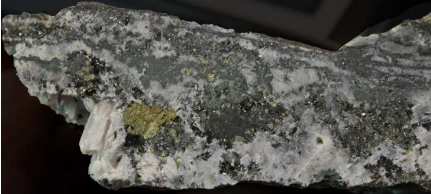
Dundok No 2 Adit Dump. Sample 155897. Banded magnetite-specularite-pyrite-pyrrhotite vein, with slabby shingle breccia vein wall margin and late-stage open cavity vugh infill with coarse dog tooth quartz vugh and coarse-grained chalcopyrite.
