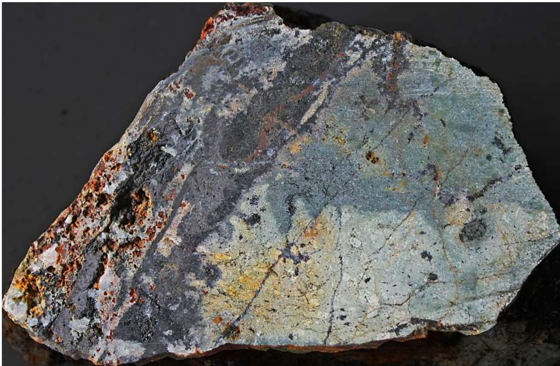
Haman Project – E Vein area. Sample 242739-5: 0.04g/t Au, 0.11% Cu, 22ppm Ga, 11.00% Fe. Quartz-specular hematite-magnetite vein at contact of acid-intermediate dyke with diffuse, uneven boundary in siltstone. Vein quartz is zonal with abundant cavities lined with goethite. The dyke contains 1-3mm size feldspar phenocrysts set in a finer grained matrix of feldspars, suggesting the dyke was dacitic in composition. Magnetite infills fractures in the dacite, with “dusting” suggesting calc-potassic alteration.
