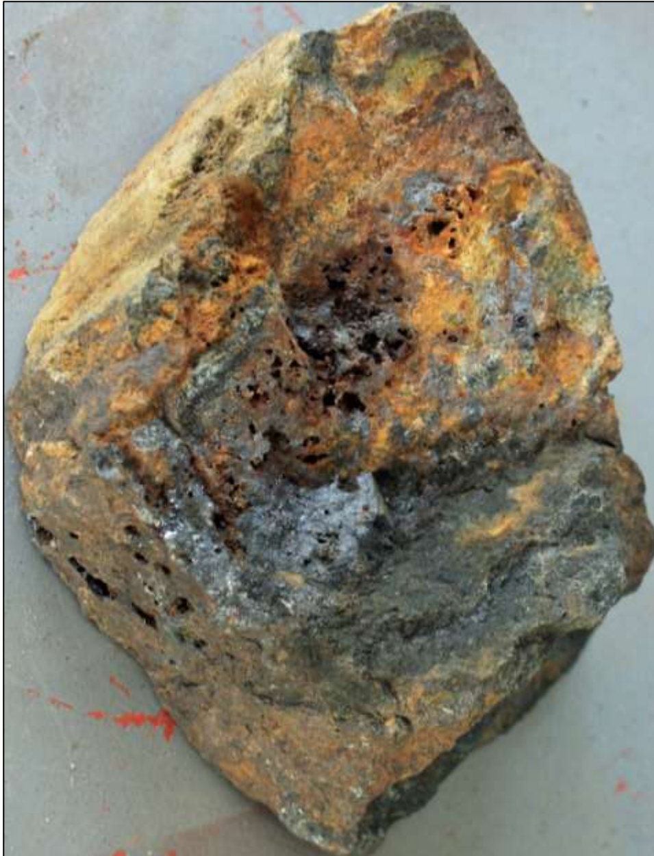
Haman Project – C Vein area. Sample 242738: 0.17g/t Au, 352ppm As, 25ppm Ga, 261ppm Mo, 11ppm Sb, 1.3ppm Te, 20.80% Fe. Magnetite-sulphide skarn, jarosite-goethite stained with cavities.
