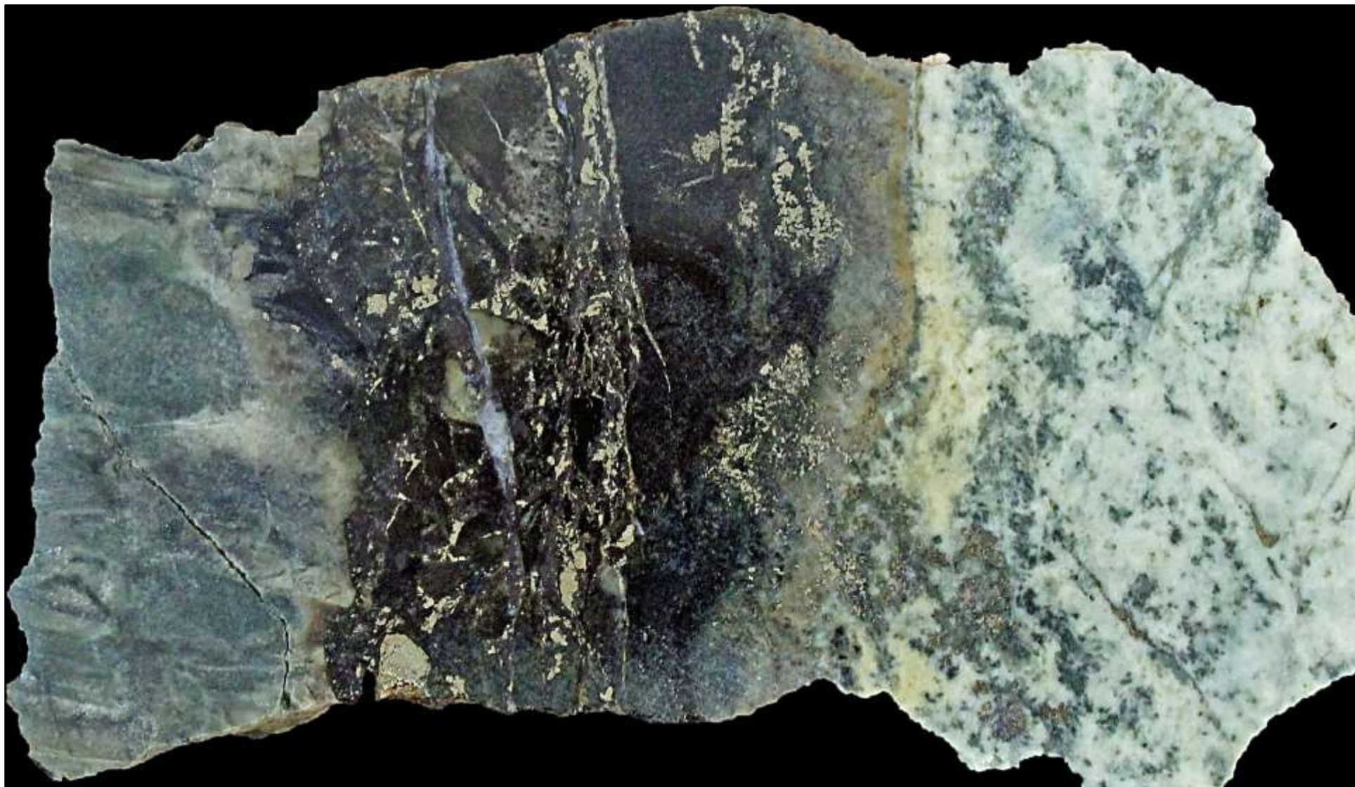
Multi-phase banded vein, Ilkwang No 2 Adit. Sample 155892: 2.04g/t Au, 6g/t Ag, 0.95% Cu, 24ppm Ga, 139ppm Ni, 174ppm Co, 101ppm V & 14.25% Fe. The vein consists of hornfels/silicified sediment at left with diffuse vein wall contact of cloudy white comb quartz apparently replacing and assimilating along porous bedding planes. The vein margin at right consists of white, "jigsaw textured" quartz (recrystallized quartz after original amorphous quartz) containing trails and disseminations of sulphides. The banded core of the vein is composed of late-stage deposition of specular hematite, magnetite and sulphides.
