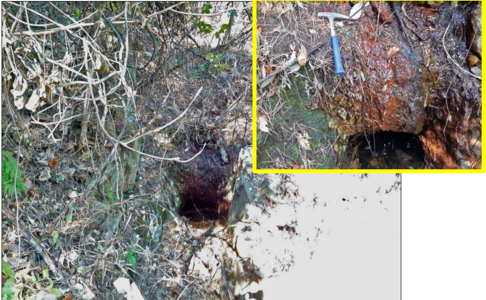
Ilkwang No 1 Adit, Jaeilgunbuk workings. Inset shows close up of the vein structure exposed in roof of this water-filled adit, with minor acid-mine drainage seepage.
