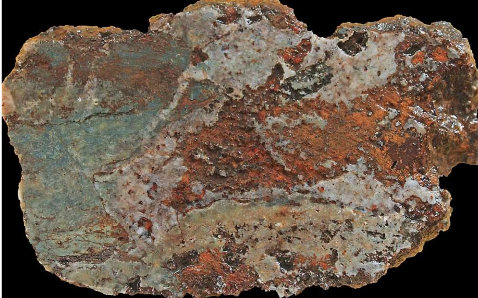
Jaeilgunbuk - Ilkwang Adit dump. Sample 242732-1: 0.56g/t Au, 3g/t Ag, 0.55% Cu, 18ppm Ga, 21ppm Mo, 0.30% Mn, 0.10% P, 12.25% Fe, 144ppm V. Quartz vein with cavities infilled with soft, porous hematite-goethite, hosted in epidote-chlorite altered siltstone. The quartz displays zonal prismatic quartz crystals, with cavities between crystals originally infilled with specular hematite-sulphide.
