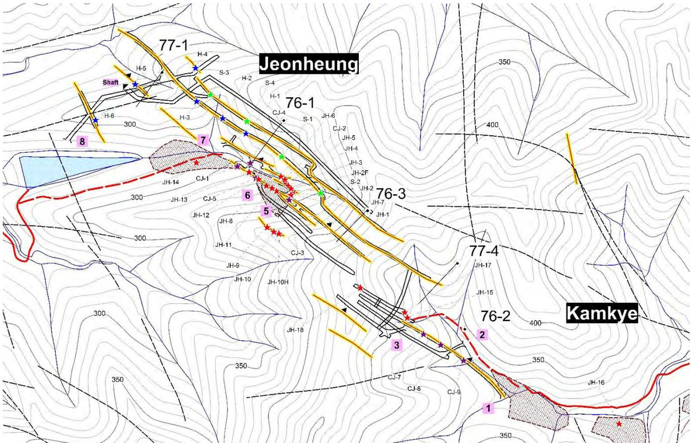
Surface Projection of the Jeonheung-Kamkye Mine Workings, with underground sample locations and drill holes.
