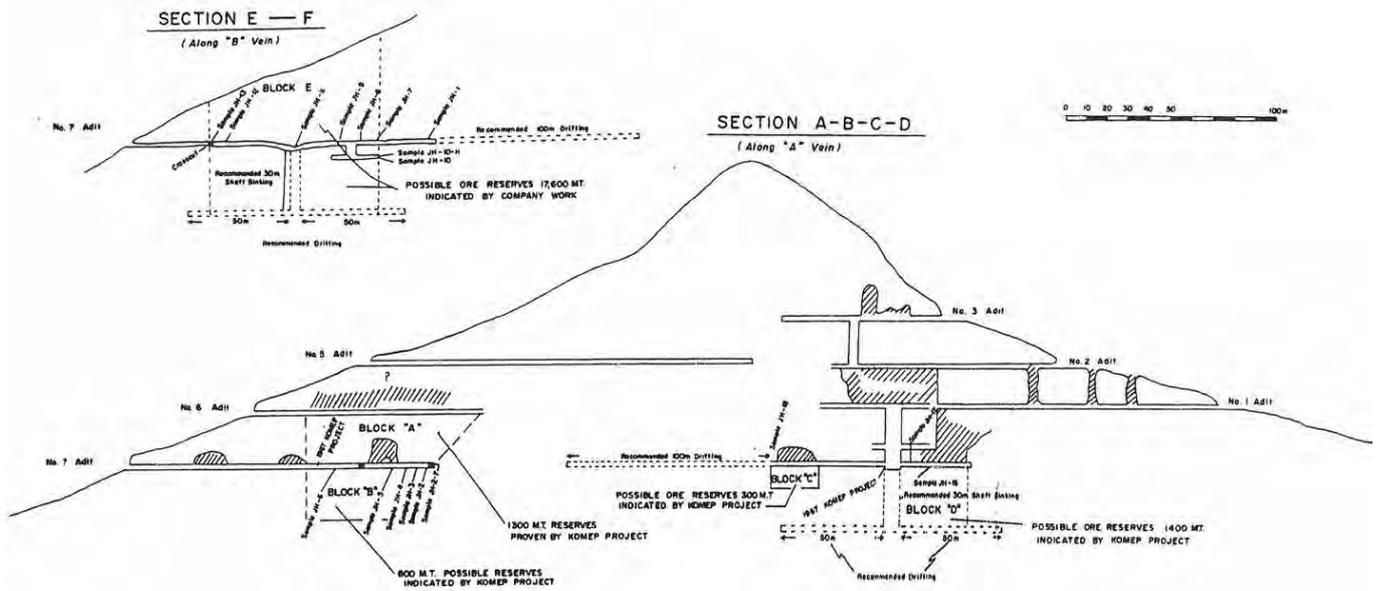
Long Section of the Jeonheung-Kamkye Mine Workings, with sampling and estimated resources prior to commencement of mining operations (after KMPC, 1978). The hatched area is the mined stopes.
