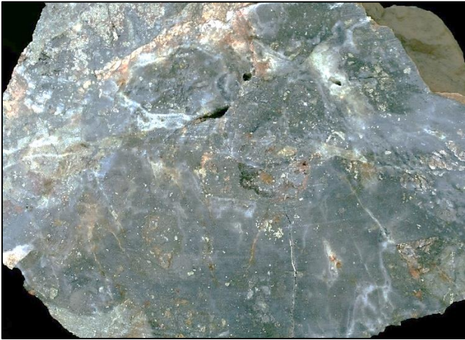
Cut slab of quartz-carbonate vein and siliceous breccia from the KeumdongChilbo No 1 dump. Sample No 242724; 1.37g/t Au, 37.4g/t Ag, 648ppm Cu, 0.78% Pb, 4.99% Zn, 326ppm Sb, 131ppm Mo, 1.93% As & 8.00% Fe as pyrrhotite.
