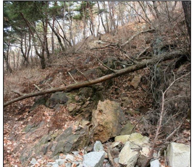
View looking north along the 3m wide slot excavated along the breccia vein structure at the Goroseoksan mine. A 4m wide, low-grade intense silica-sericite-sulphide alteration zone is developed in the unmined hangingwall at left.
