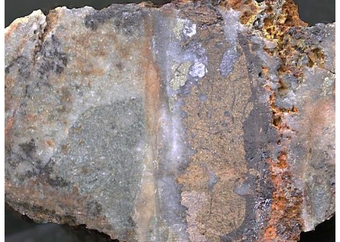
Early dark grey-brown Fe-rich sphalerite cut by later honey yellow Fe-poor sphalerite, Keumdongchilbo. Sample 242721: 0.60g/t Au, 94g/t Ag, 2.42% Pb, 1.66% Zn, 344ppm Cu, 0.39% As, 65ppm Bi, 152ppm Sb, 102ppm In, 0.11% Cd.
