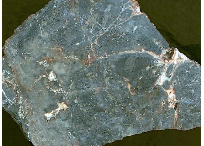
Hydrothermal breccia overprinted by jigsaw quartz-adularia vein-vugh infill, Keumdongchilbo. Sample 242728: 0.78g/t Au, 201g/t Ag, 0.14% Cu, 4.32% Pb, 5.61% Zn, 782ppm Sb, 45ppm Mo, 534ppm Cd, 1.14% As.
