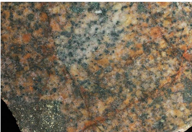
Silica-actinolite-sulphide altered monzonite, with pale orange-brown hematite dusting of feldspars indicative of calc-potassic sodic alteration, KeumdongChilbo prospect. Sample No 242721b; 3g/t Ag, 660ppm Ba, 409ppm Pb, 435ppm Zn, & 18ppm Sb
