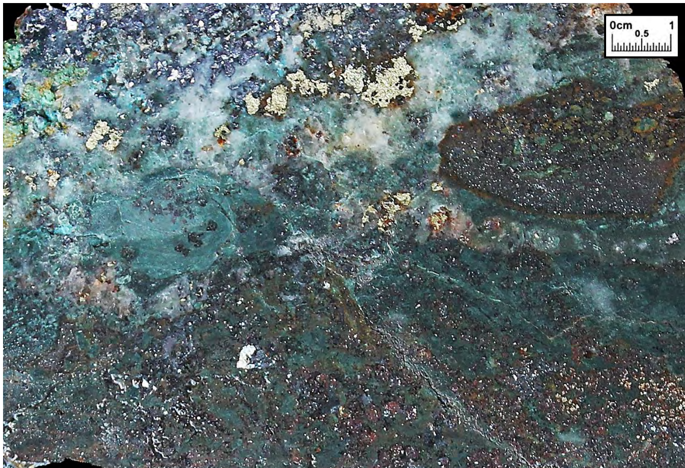
Weakly developed banding comprising comb quartz vein stockwork with chalcopyrite and breccia of sphalerite-galena, is hosted in sericite-chlorite (blue-green)-specular hematite-smectite clay altered siltstone. A thin chill margin of Fe-chlorite lines the quartz veining. Hwangsan No 2 mine dump. Sample 155579: 0.11g/t Au, 140g/t Ag, 0.90% Cu, 2.31% Pb, 2.82% Zn, 0.147% Mo, 388ppm Bi, 215ppm W, 185ppm As.
