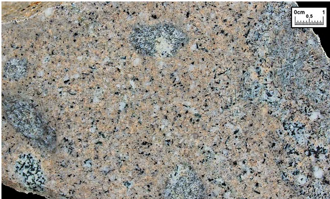
Sample 243475. Medium-grained monzogranite at Hwanghaksan mountain (3km east of Ogsan). Note the entrained xenoliths of an early, more mafic and finer-grained phase.
