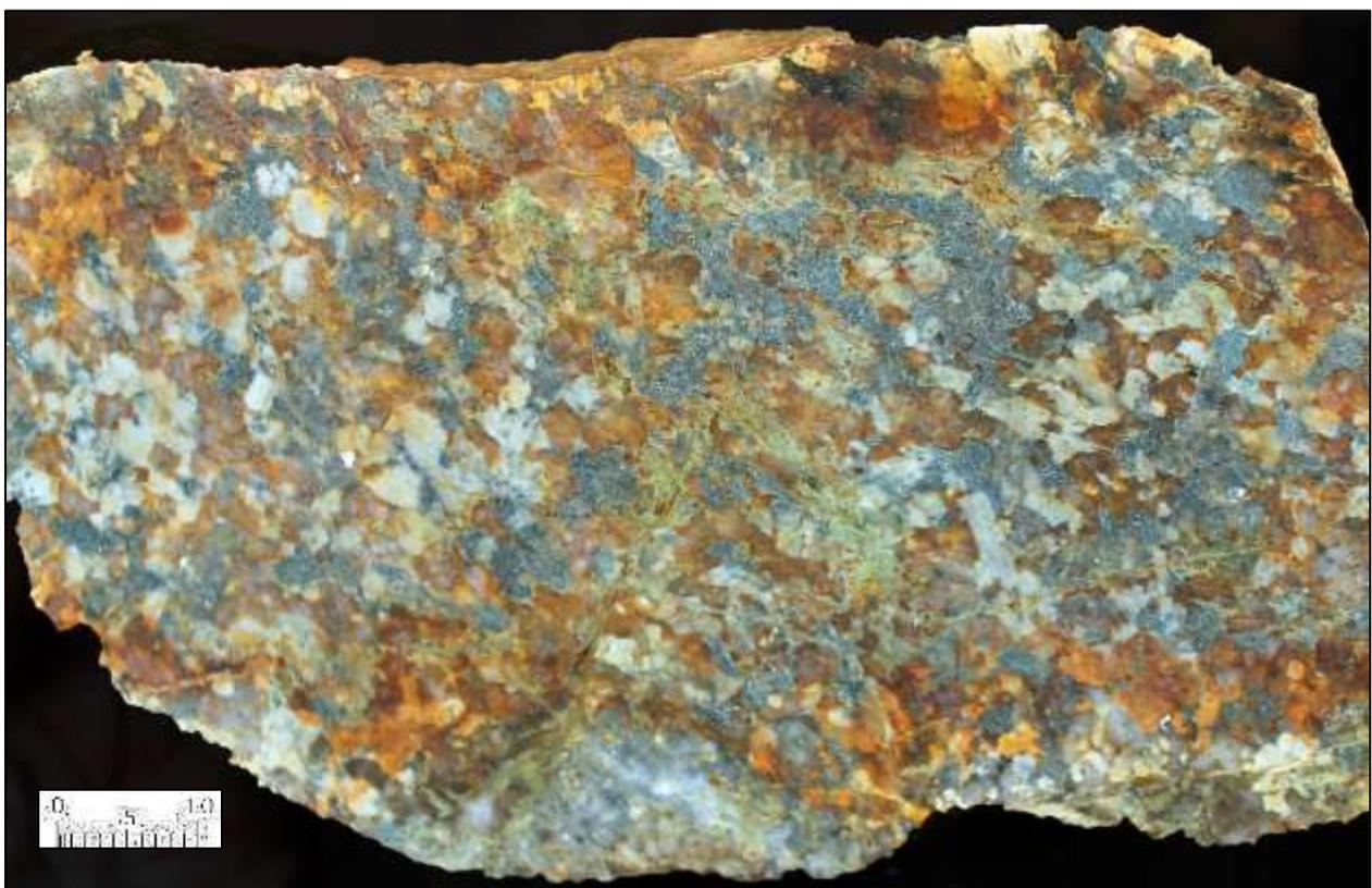
Photograph 34. Cut slab of limonite stained, oxidized sericite-jarosite altered coarse-grained granite gneiss. Anomaly F, Sample no 243275.
