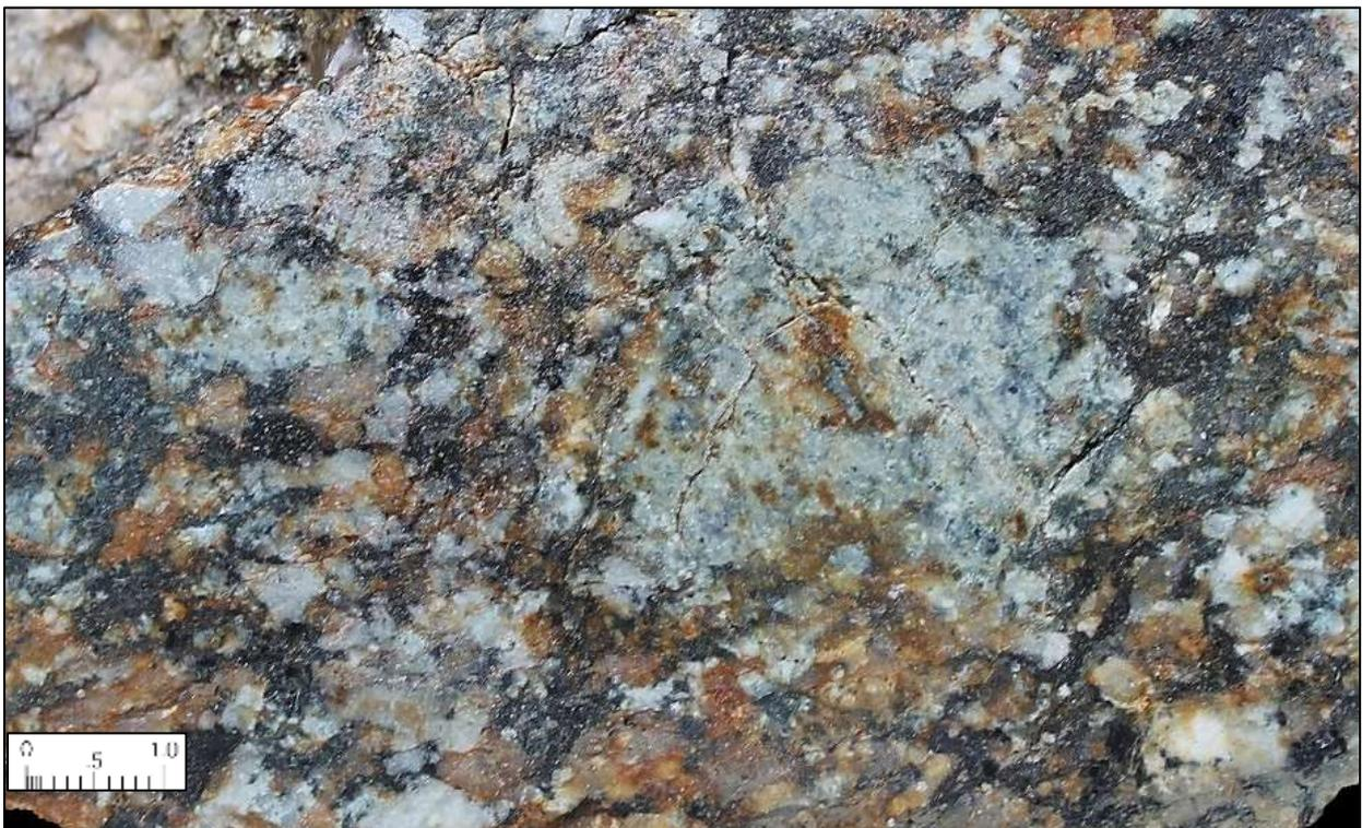
**Photograph 10. Cut slab of coarse-grained porphyroblastic granite gneiss, with dark biotite micas, quartz, white plagioclase and pink k-feldspar grains. Plagioclase feldspar has been altered to zoisite, chlorite, amphibole and carbonate (saussurite assemblage). Limonite staining. Sample no 243428.**
