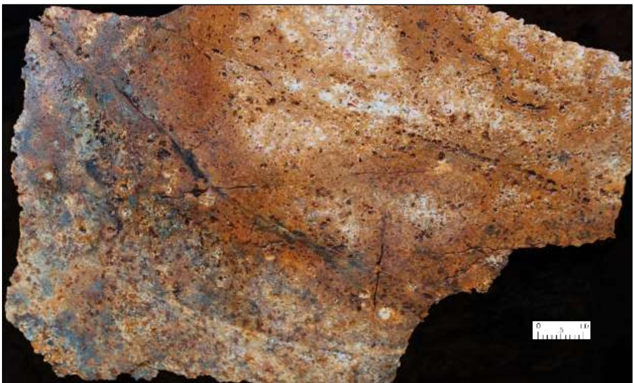
Photograph 30. Cut slab of leached, gossanous, porous, brecciated mineralized diorite porphyry. Anomaly F, Sample No 243281 (46g/t Ag, 0.11% Cu).
