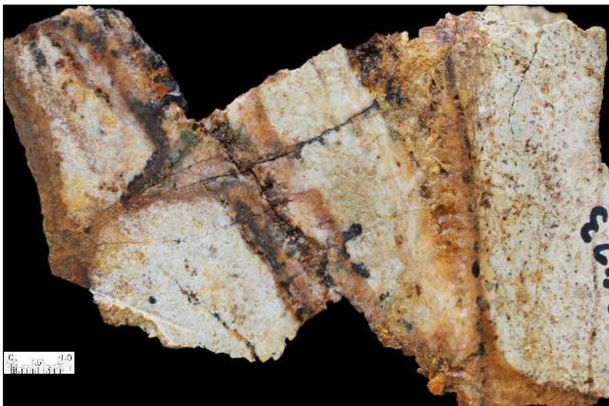
Photograph 25. Cut slab of gossanous quartz vein-fracture stockwork in leached, porous, brecciated diorite porphyry. Anomaly I, Sample no 243423 (8g/t Ag, 0.13% Cu, 0.30% Pb & 0.14% Zn).
