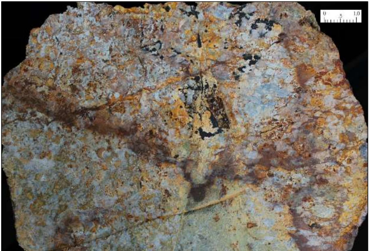
Photograph 29. Cut slab of leached, brecciated, sericite altered, coarse-grained granite gneiss. Anomaly B, Sample No 243419 (41g/t Ag, 0.13% Cu, 0.22% Pb & 0.12% Zn).
