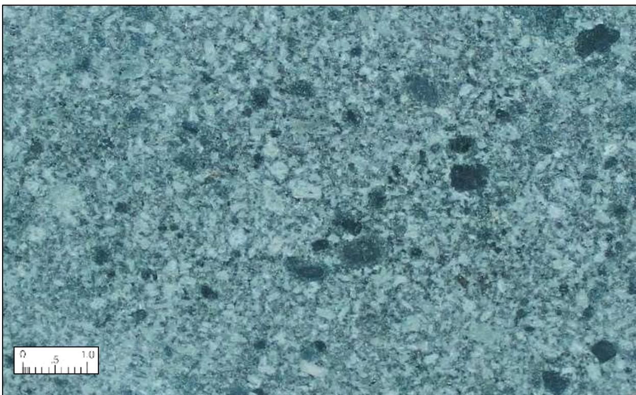
Photograph 15. Cut slab of blue-tinged uralite (deuteric alteration) and chlorite altered porphyritic andesite tuff. Sample no 243425. Abundant xenoliths of fine sediments are evident (dark grey clasts) within a densely packed, poorly sorted mass of inequigranular grains of feldspar, quartz and mafics.
