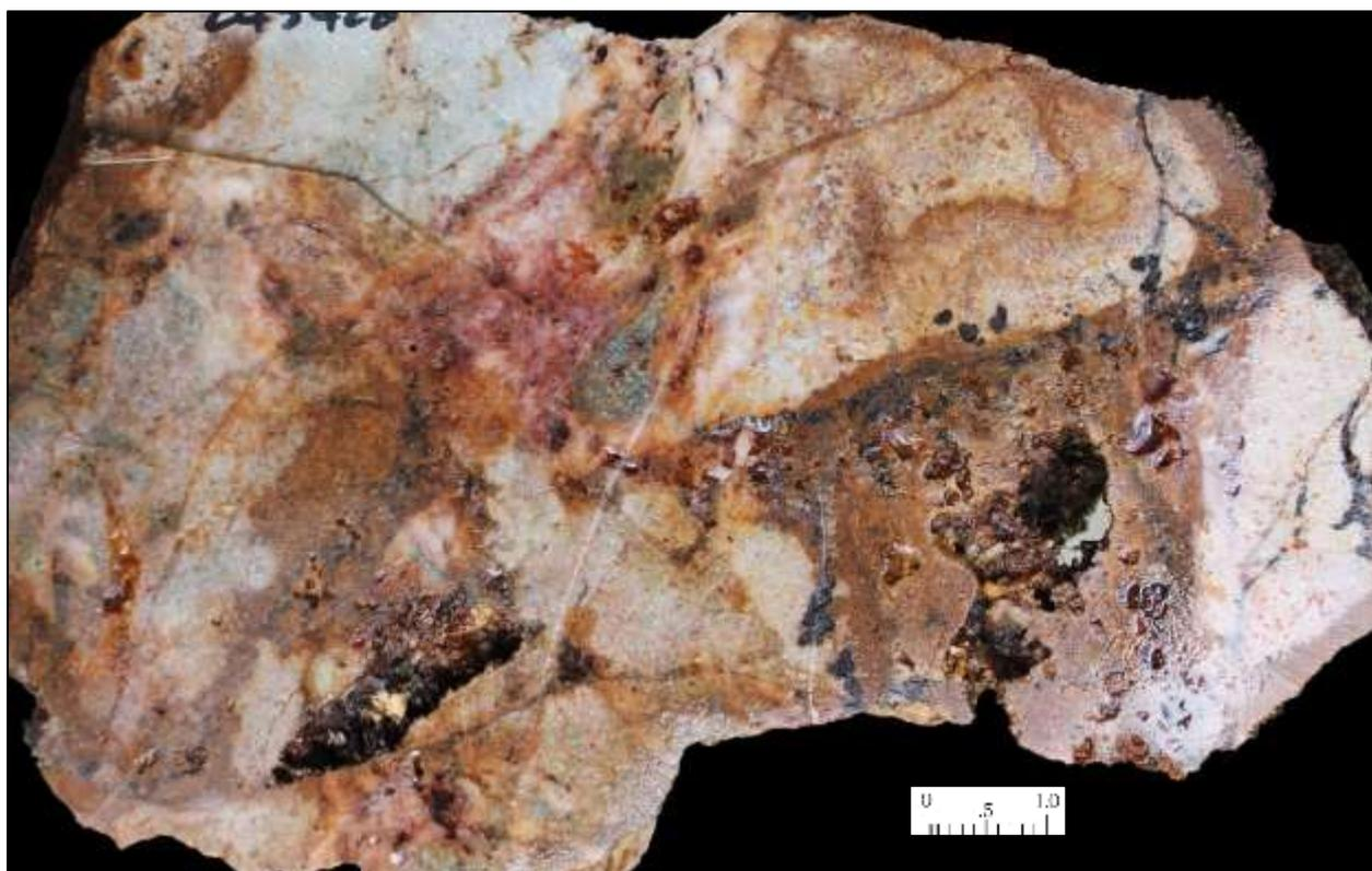
Photograph 26. Cut slab of leached, porous breccia composed of diorite porphyry and granite gneiss clasts cemented by a vuggy matrix infill of quartz and gossan after sulphides. The clasts display diffuse embayed and corroded margins. Anomaly I, Sample no 243426 (9g/t Ag, 840ppm Cu, 0.20% Pb & 0.14% Zn).
