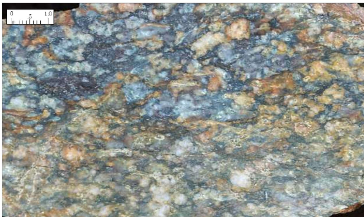
Photograph 11. Cut slab of coarse-grained porphyroblastic textured granite gneiss. Myrmekitic quartz vermicule texture is commonly developed within the plagioclase (albite) grains. Sample no 243284.
