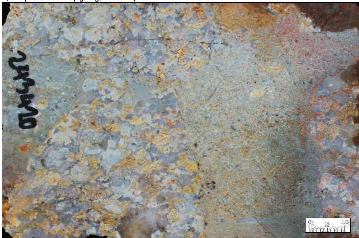
Photograph 24. Cut slab of limonite stained, brecciated, sericite altered, coarse-grained granite gneiss. Anomaly B, Sample No 243420 (0.15% Pb).
