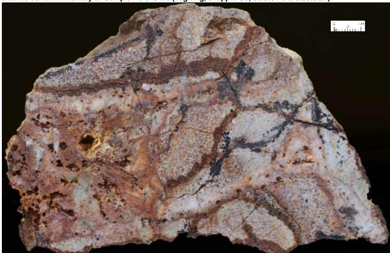
Photograph 28. Cut slab of leached, porous, brecciated mineralized diorite porphyry, with gossanous matrix. Anomaly I, Sample No 243427 (8g/t Ag, 0.12% Cu, 0.20% Pb & 0.15% Zn).
