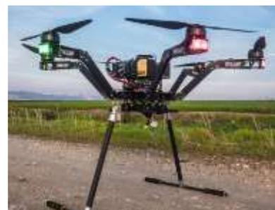
Flying at low altitude (30m) with the bird on a 10m tow line, at a minimum speed of 10m/s to minimize drag, a c-drone UAV can cover ground 6-10 times faster than a walking operator, in all types of terrain, be flown at night, in poor visibility conditions, and over dangerous topography.
