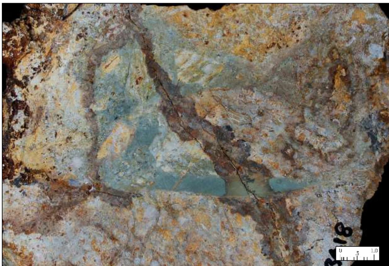
Photograph 27. Cut slab of breccia dominated by gossanous granite gneiss clasts within a matrix of fine silica-chlorite cement. Anomaly B. Sample No 243418 (10g/t Ag, 518ppm Cu, 0.28% Pb & 0.23% Zn).
