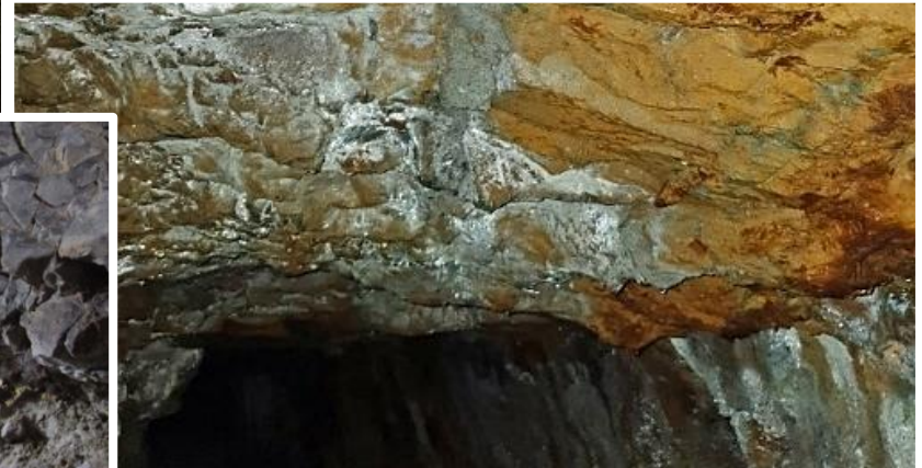
Vein-breccia exposed in roof of Seongji Adit
