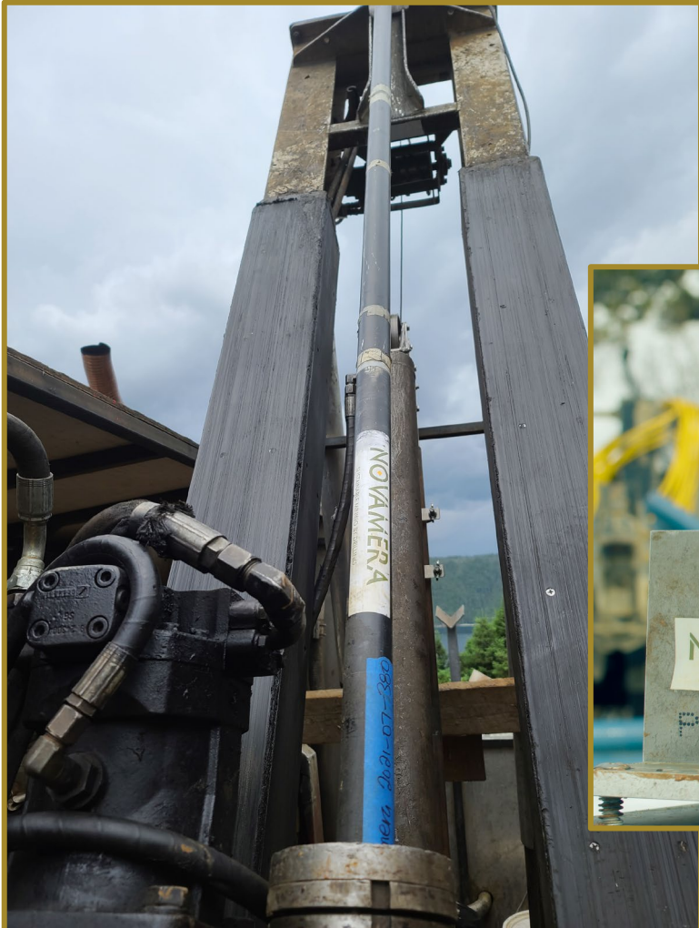
NBIT deployed in core drill
